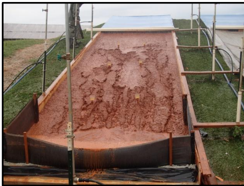
Figure 10. Type B Silt Fence End-of-Test
