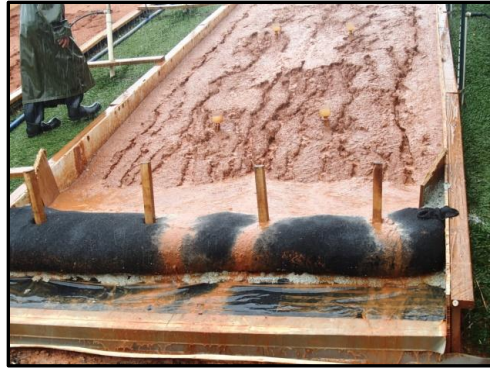
Figure 9. Type B Compost Sock End-of-Test
