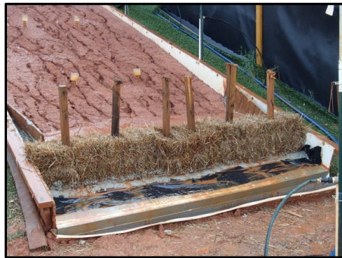
Figure 11. Type B Straw Bales End-of-Test
