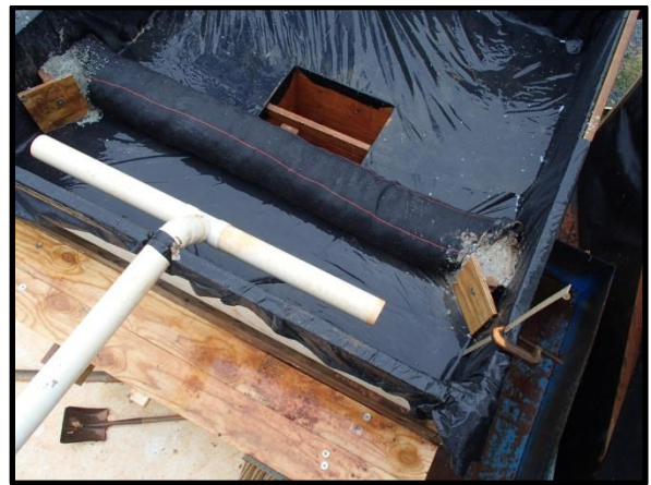
Figure 6. Paved Test Setup – GSWCC Sd2-P (Wrapped Stone)
