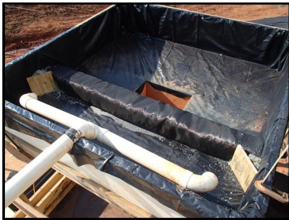
Figure 5. Paved Test Setup – GSWCC Sd2-P (Pigs-In-A-Blanket)
